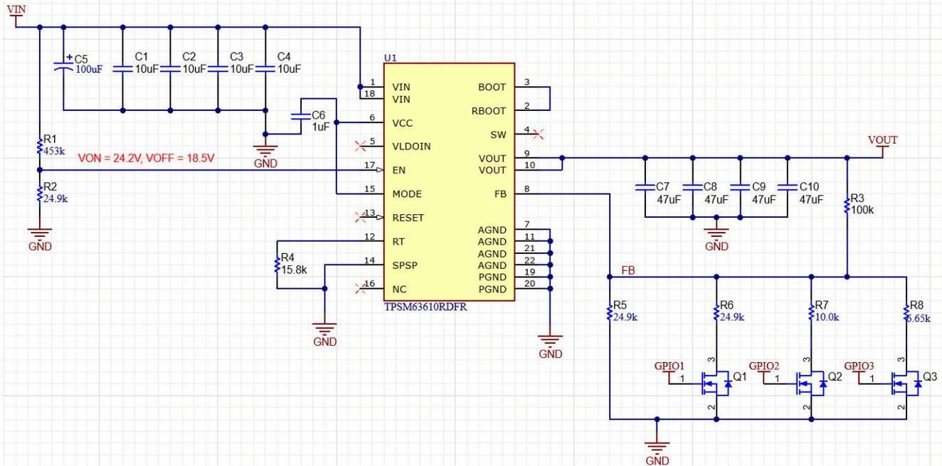
**Figure 4-1. USB Type-C Schematic Using the TPSM63610 Power Module with Feedback Resistor Network Control**
