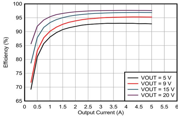
Figure 5-1. Efficiency Measurement for  $V_{IN} = 24\text{-V}$
