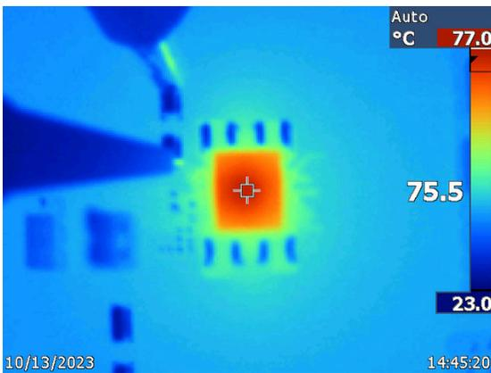
Figure 5-5. Thermal Measurement for  $V_{OUT} = 15\text{-V}$
