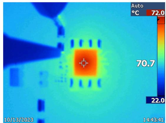
Figure 5-4. Thermal Measurement for  $V_{OUT} = 9\text{-V}$
