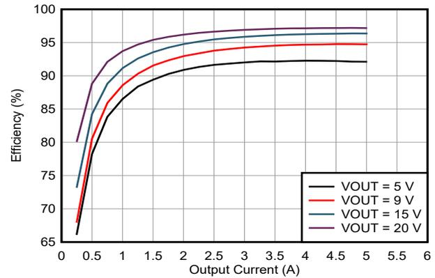
Figure 5-2. Efficiency Measurement for  $V_{IN} = 28\text{-V}$
