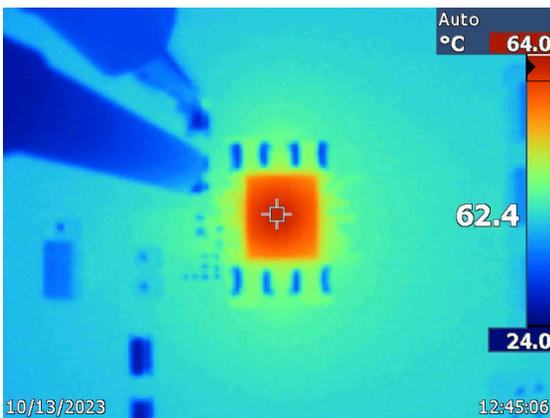
Figure 5-3. Thermal Measurement for  $V_{OUT} = 5\text{-V}$
