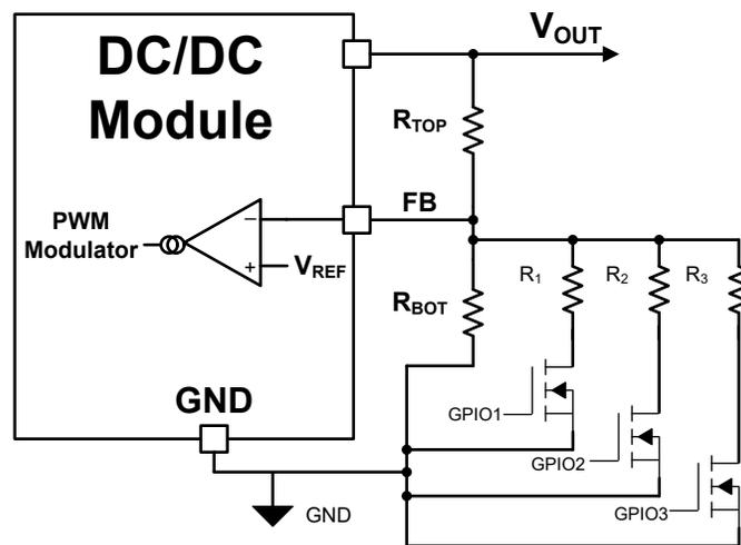
**Figure 3-1. Feedback Resistor Switch Network Control Scheme**
