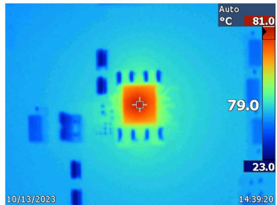
Figure 5-6. Thermal Measurement for  $V_{OUT} = 20\text{-V}$
