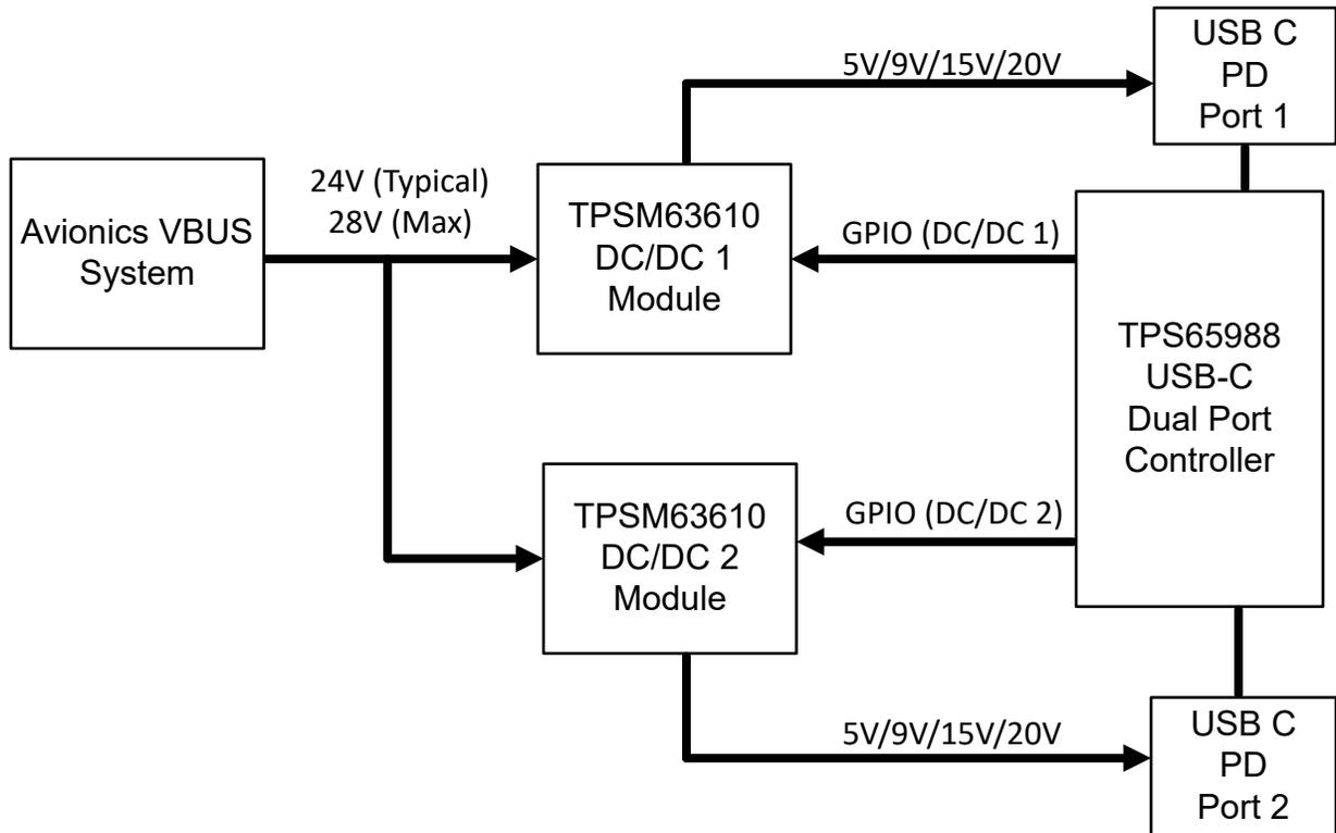
Figure 2-1. Dual-Port USB Type-C Power/Data Source
