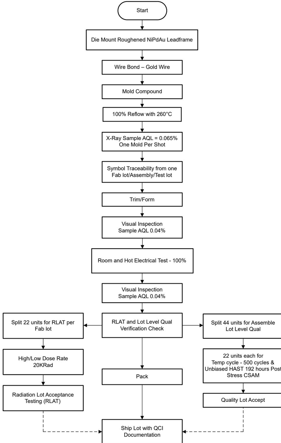
**Figure 2-1. TPS7H4010-SEP Space Enhanced Plastic Production Flow Chart**
