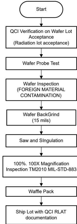
**Figure 2-2. TPS7H4010-SEP Space Enhanced KGD Production Flow Chart**
