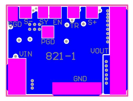
Figure 24. Bottom Copper and Paste Layers (Bottom view)
