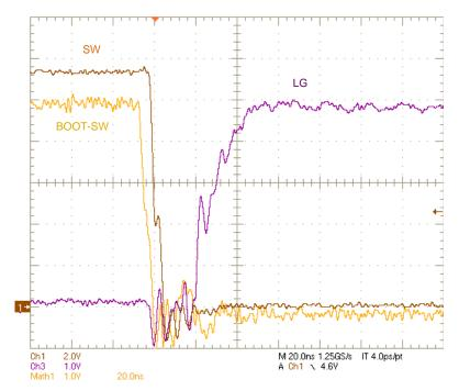
Figure 18. Deadtime Prior To High-side MOSFET Turn-off;  $V_{IN}$  = 12 V,  $V_{OUT}$  = 1.8 V, 120-m $\Omega$  Load
