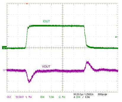
Figure 9. Load Transient Response;  $V_{IN} = 12 V$ ,  $V_{OUT} = 1.8 V$ , 0 A to 10 A at 2 A/µs
