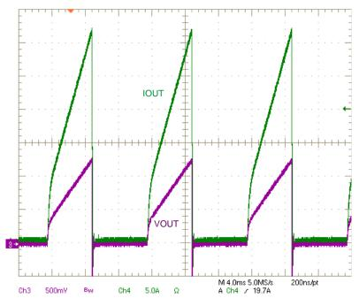
Figure 8. Current Limit Hiccup Mode
