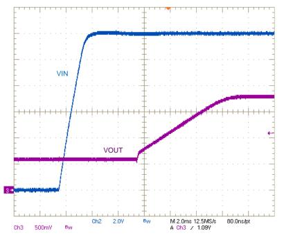
Figure 15. Pre-bias Startup;  $V_{IN}$  = 12 V, No Load, 0.6-V Pre-bias
