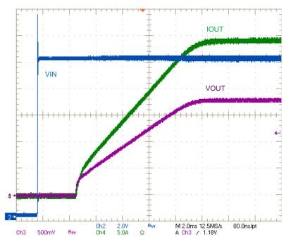
Figure 11. Startup with VIN Stepped to 12 V; V<sub>out</sub> = 1.8 V, 30-A Resistive Load
