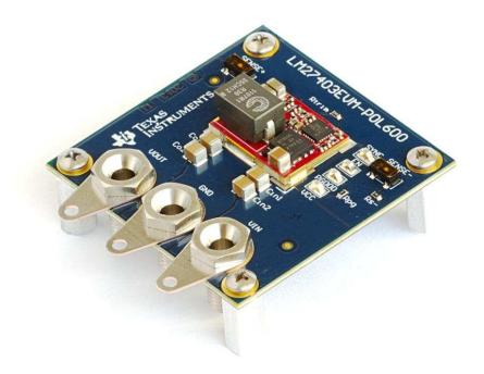
Figure 3. Photo of Module SMT Connected to Host PCB
