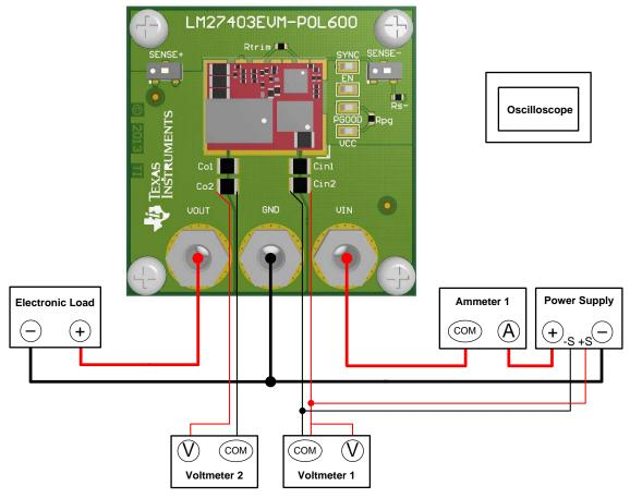
Figure 4. Connection Diagram
