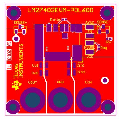
Figure 25. Top Copper and Paste Layers
