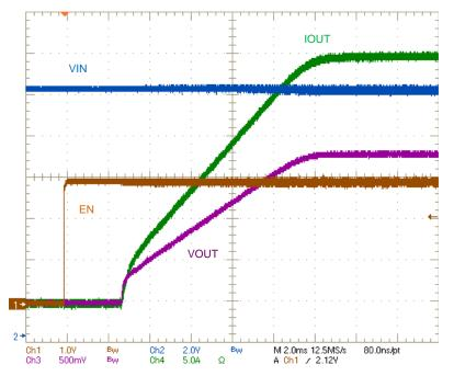
Figure 13. Startup with EN Stepped to 3 V;  $V_{IN}$  = 12 V,  $V_{OUT}$  = 1.8 V, 30-A Resistive Load
