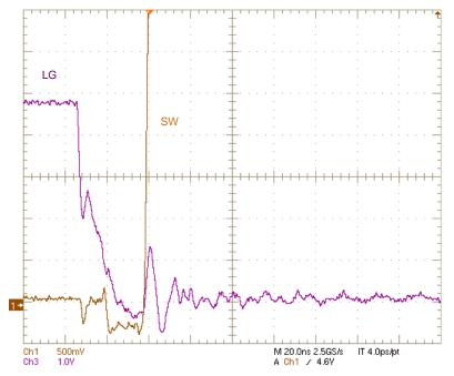
Figure 17. Deadtime Prior To High-side MOSFET Turn-on; V<sub>IN</sub> = 12 V, V<sub>OUT</sub> = 1.8 V, 120-mΩ Load
