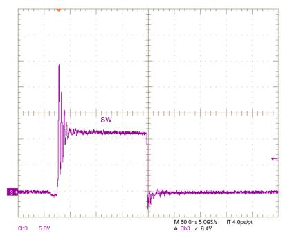
Figure 16. Switch Node Voltage;  $V_{IN}$  = 12 V,  $V_{OUT}$  = 1.8 V
