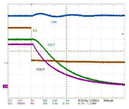
Figure 14. Shutdown with EN Pulled To GND;  $V_{IN}$  = 12 V,  $V_{OUT}$  = 1.8 V, 20-A Resistive Load
