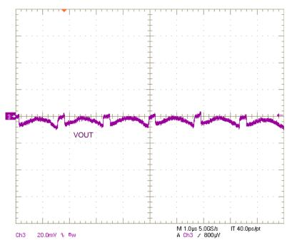
Figure 10. Output Voltage Ripple;  $V_{IN} = 12 V$ ,  $V_{OUT} = 1.8 V$ ,  $I_{OUT} = 20 A$
