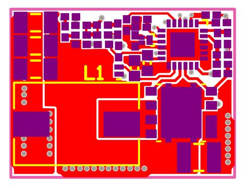
Figure 21. Top Copper and Paste Layers
