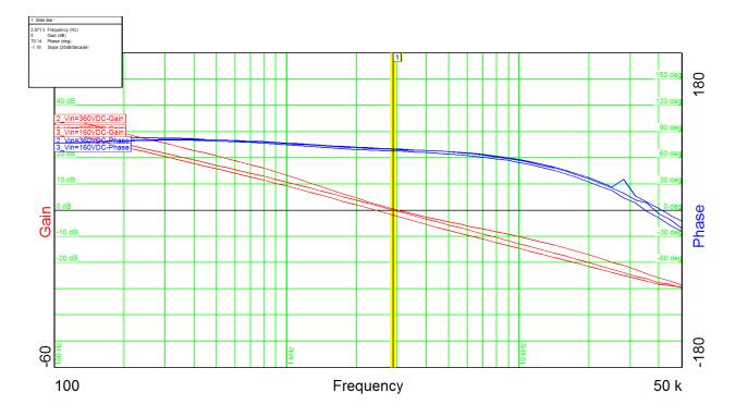
$\begin{array}{ll} \text{Output power} & = 5 \text{V} @ 2.1 \text{A} \\ \text{Input voltage} & = 160 \text{VDC} \\ \text{Phase margin} & = 68^{\circ} \\ \text{Bandwidth} & = 2.4 \text{kHz} \end{array}$
