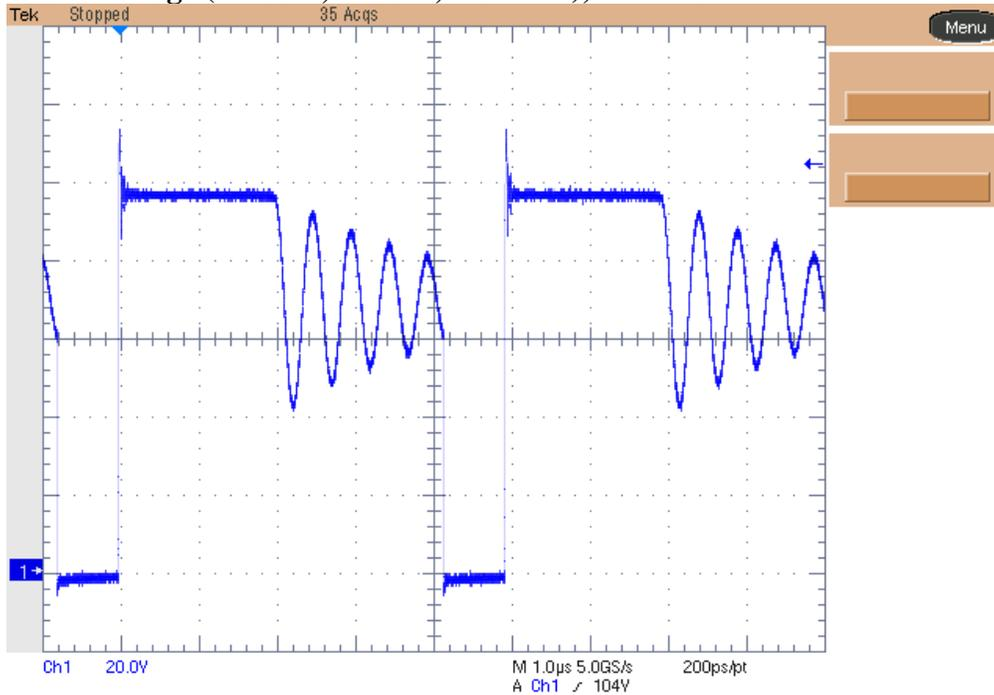
**Ch1: Q1 drain Voltage (20V/div, 10us/div, No BWL), 50mA load, Burst mode operation**
