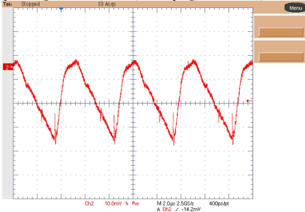
**Ch.2: Output Voltage (20mV/div, 20us/div, AC coupling, 20MHz BWL), I<sub>out</sub> = 100mA**
