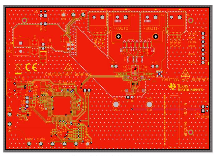
Figure 4. TPS65653-Q1 Board Layout
