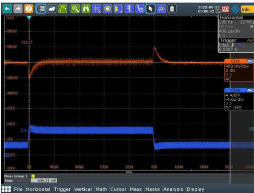
Figure 3-20. Load Step ( $V_{IN} = 16V$ ,  $I_{OUT} = 2A - 5A$ )
