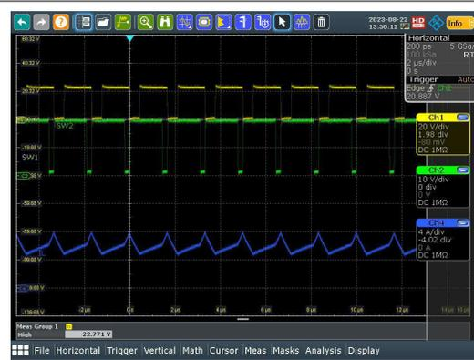
Figure 3-15. SW1, SW2,  $I_L$  ( $V_{IN} = 24V$ ,  $I_{OUT} = 5.0A$ )
