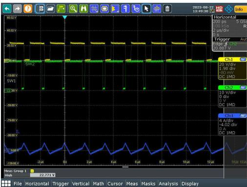
Figure 3-12. SW1, SW2,  $I_L$  ( $V_{IN} = 16V$ ,  $I_{OUT} = 0A$ )
