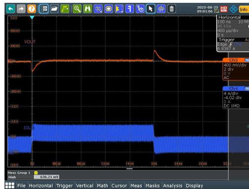
Figure 3-22. Load Step ( $V_{IN} = 36V$ ,  $I_{OUT} = 2A - 5A$ )
