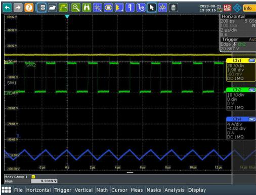
Figure 3-8. SW1, SW2,  $I_L$  ( $V_{IN} = 9V$ ,  $I_{OUT} = 0A$ )
