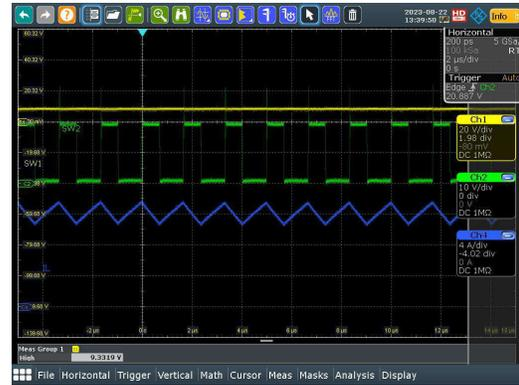
Figure 3-9. SW1, SW2,  $I_L$  ( $V_{IN} = 9V$ ,  $I_{OUT} = 5.0A$ )
