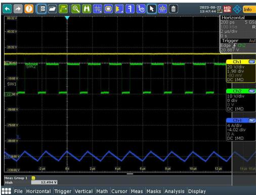
Figure 3-10. SW1, SW2,  $I_L$  ( $V_{IN} = 12V$ ,  $I_{OUT} = 0A$ )
