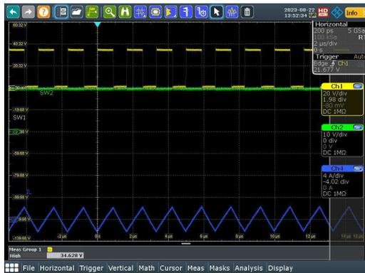
Figure 3-16. SW1, SW2,  $I_L$  ( $V_{IN} = 36V$ ,  $I_{OUT} = 0A$ )
