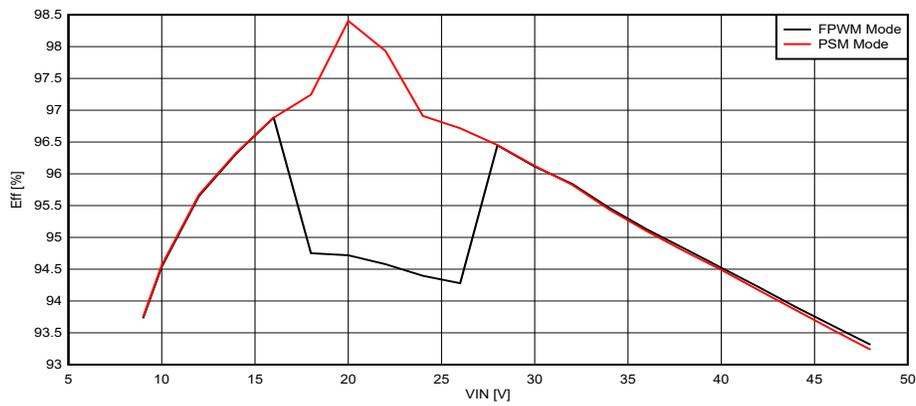
Figure 3-7. Efficiency vs. Input Voltage,  $V_O = 20V$ ,  $I_O = 5A$
