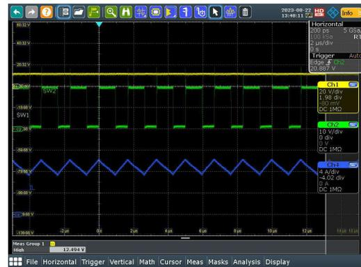
Figure 3-11. SW1, SW2,  $I_L$  ( $V_{IN} = 12V$ ,  $I_{OUT} = 5.0A$ )
