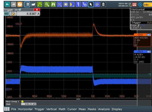
Figure 3-19. Load Step ( $V_{IN} = 12V$ ,  $I_{OUT} = 2A - 5A$ )
