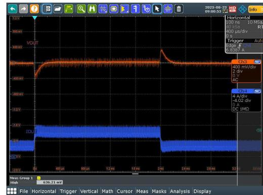
Figure 3-21. Load Step ( $V_{IN} = 24V$ ,  $I_{OUT} = 2A - 5A$ )
