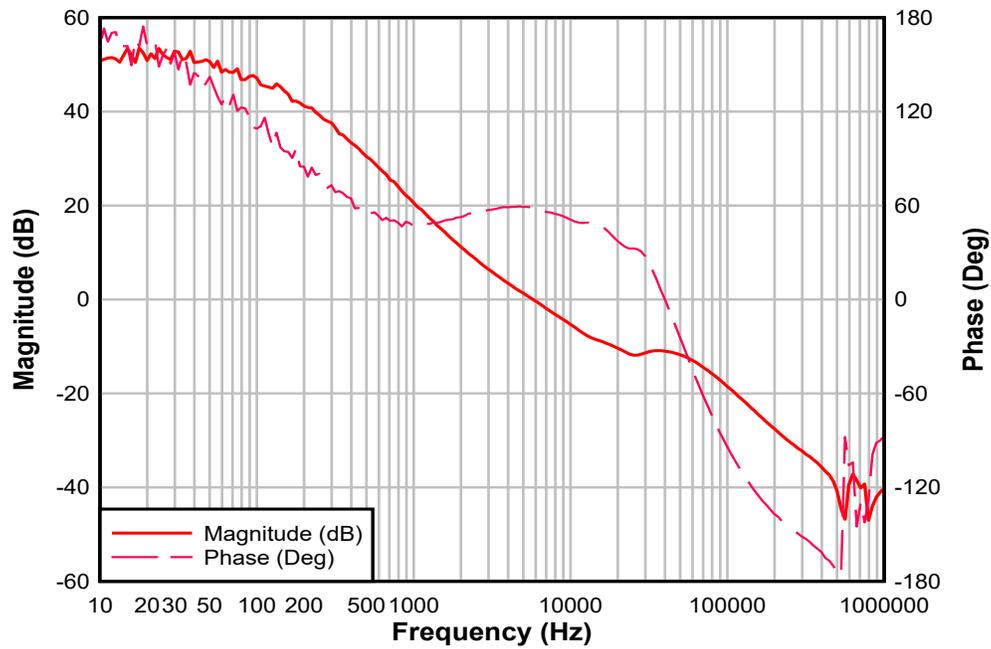
Figure 3-23. Control Loop Response, VIN = 9.0V, IOU = 5.0A
