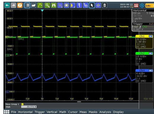
Figure 3-13. SW1, SW2,  $I_L$  ( $V_{IN} = 16V$ ,  $I_{OUT} = 5.0A$ )
