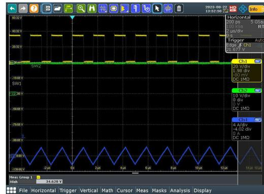
Figure 3-17. SW1, SW2,  $I_L$  ( $V_{IN} = 36V$ ,  $I_{OUT} = 5.0A$ )
