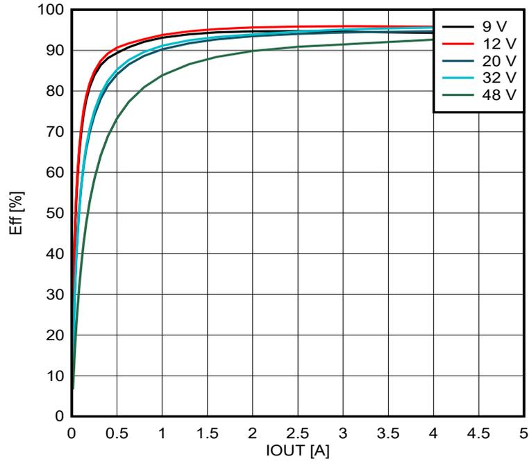
Figure 3-6. Efficiency vs. Output Current,  $V_O = 20V$
