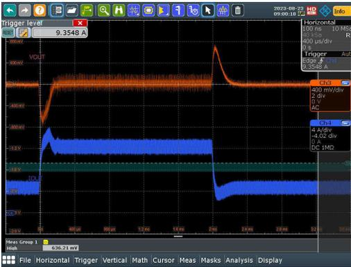
Figure 3-18. Load Step ( $V_{IN} = 9V$ ,  $I_{OUT} = 2A - 5A$ )
