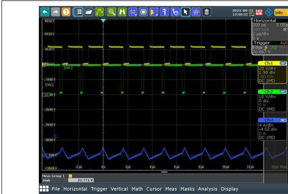
Figure 3-14. SW1, SW2,  $I_L$  ( $V_{IN} = 24V$ ,  $I_{OUT} = 0A$ )
