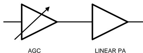
**Figure 1. Output Power Control for Linear Application**
