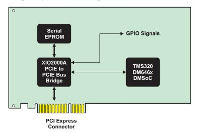
Figure 3. Bridge Adaptor Card Block Diagram
