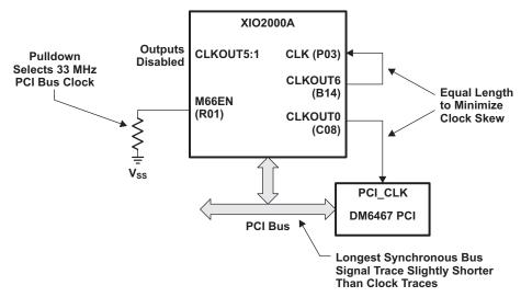
Figure 5. External PCI Bus Clock Feedback
