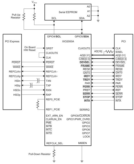
A The pullup resistors are connected to the terminals shown in bold.
