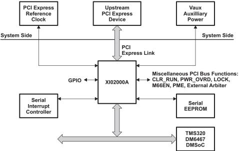
Supports Six PCI Devices: 32 Bit, 33 MHz
