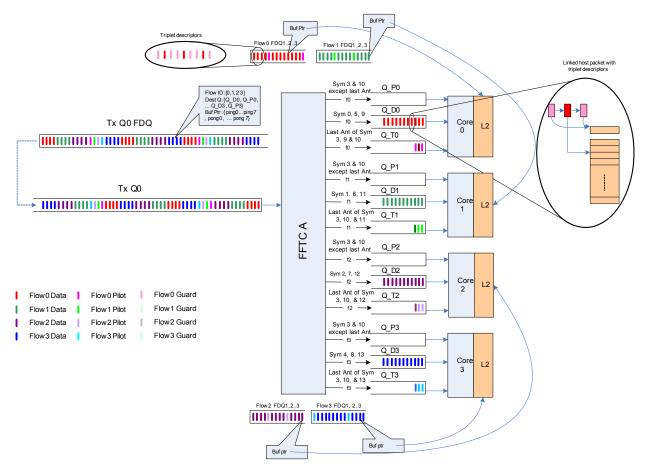
Figure 11 shows a complete picture of an example usage of LTE PUSCH and PUCCH around FFTC. It uses the single queue data path idea as described in section "6.3 Advanced Usage" on page 25 to reconstruct the packets so as to connect AIF2 and FFTC on inbound traffic.
