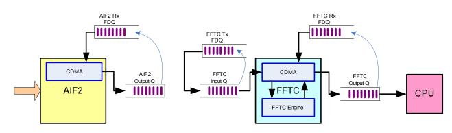
If the accumulator is used to generate the synchronization event, it can be generated when all antenna data of one OFDM symbol are received. Upon the synchronization event trigger, the following steps need be done by the EDMA either by chaining different EDMA channels or by self-chaining and linking to the same EDMA channel: 1. Copy the AIF2 PS words to the end of the FFTC PS word buffer
