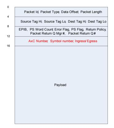
The highlighted words in red contain protocol specific (PS) data for AIF2. AIF2 can have another form of protocol specific data which contains OBSAI address and ingress/egress indication, which is beyond the scope of this application note.
