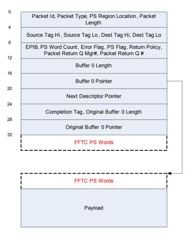
The highlighted fields are protocol-specific words, which are the same as in the monolithic packet, so it is condensed into one block for simplicity of the picture. There are two choices for where the PS words can be in host mode, at the end of the packet descriptor or at the start of payload (SOP), as shown by the dashed line rectangle boxes.
