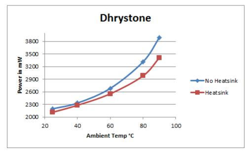
Figure 4. Power Consumption vs Ambient Temperature
