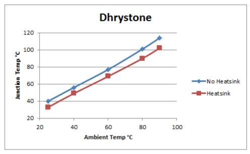
Figure 3. Junction Temperature vs Ambient Temperature
