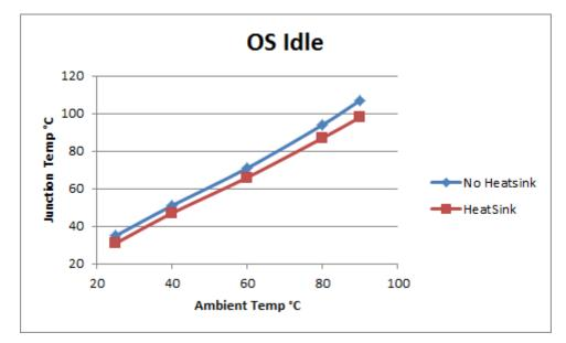
Figure 1. Junction Temperature vs Ambient Temperature
