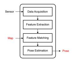
Figure 2-3. Localization Process With Pre-built Map
