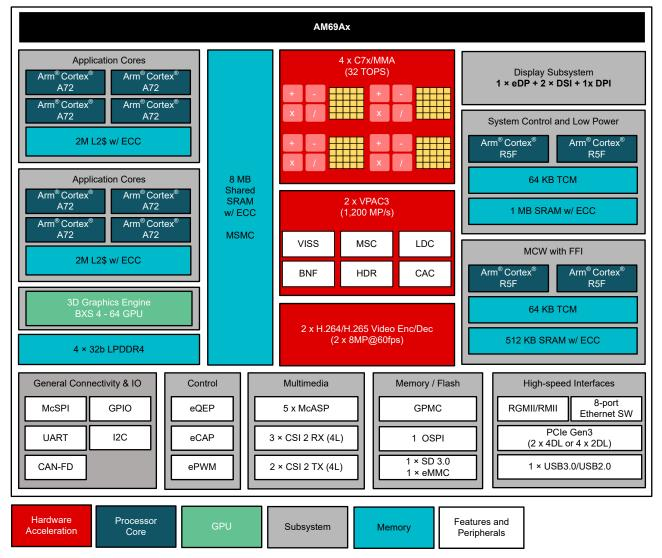
Figure 1-2. AM69A Simplified Block Diagram
