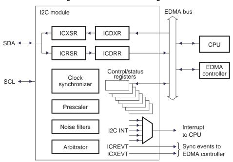
Figure 1. I2C Module Block Diagram
