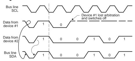
Figure 12. Arbitration Procedure Between Two Master-Transmitters
