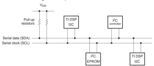
Figure 2. Multiple I2C Modules Connected
