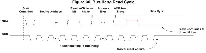
The master initiates a read in the normal fashion but a reset occurs while the SCK is high and the slave is driving the SDA low. The slave device will continue to drive SDA low waiting for the master to provide the next clock however the master has been reset and is no longer attempting to complete the read cycle. In addition, if the master attempts to access the bus after its reset has been released it will fail to arbitrate for control.
