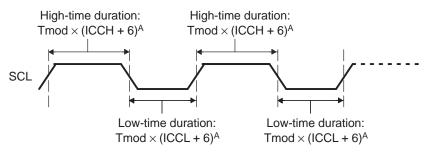
Tmod = module clock period = 1/module clock frequency
