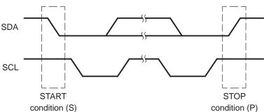
Figure 6. I2C Module START and STOP Conditions
