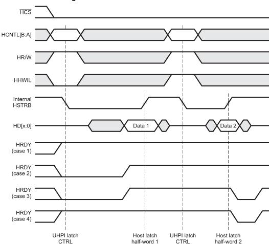
Figure 4. Host Read in Dual-Halfword Mode
