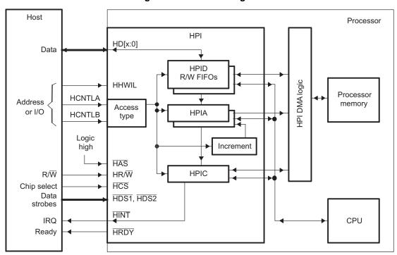
Figure 1. HPI Block Diagram
