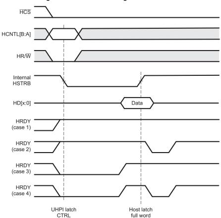
Figure 7. Host Write in Single-Fullword Mode
