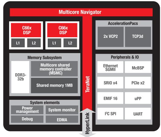
▲ Fig. 1 – TMS320C6657/55 block diagram
