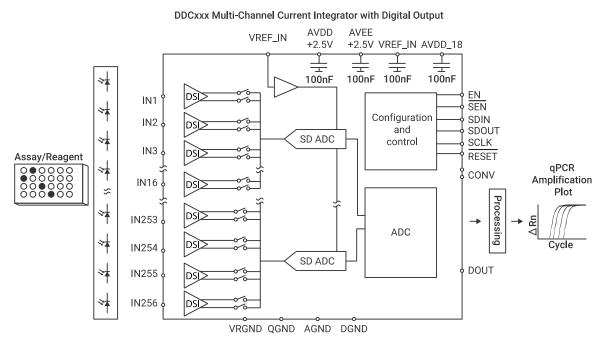
Figure 3. A DDC Integrated Optical Signal Chain for PCR
