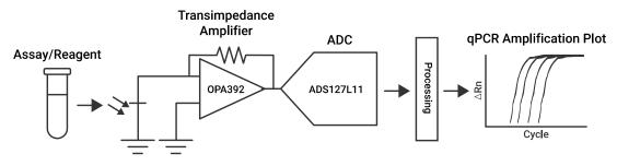
Figure 4. Discrete Optical Signal Chain for PCR
