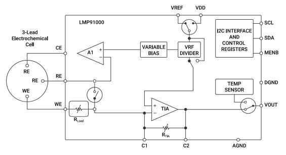
Figure 1. LMP91000 Electrochemical Cell Interface
