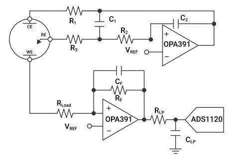
Figure 2. Discrete Electrochemical Cell Signal Chain
