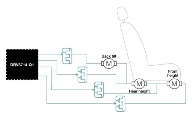
Figure 1. A Three-motor Seat Driven by the DRV8714-Q1 Automotive Gate Driver
