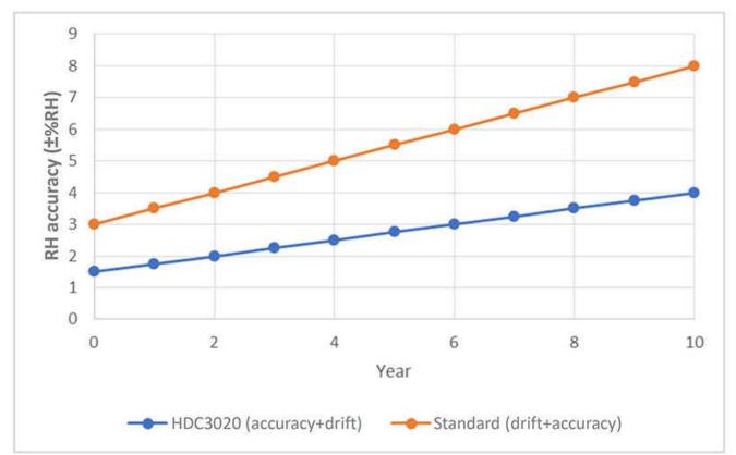
Figure 1. Humidity Sensor Accuracy with Long-term Drift
