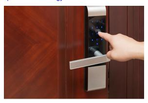
Figure 2. Touchscreen on an Electronic Lock Enabled by Capacitive Touch Technology
