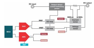
Figure 1. Typical Block Diagram of a DC Source
