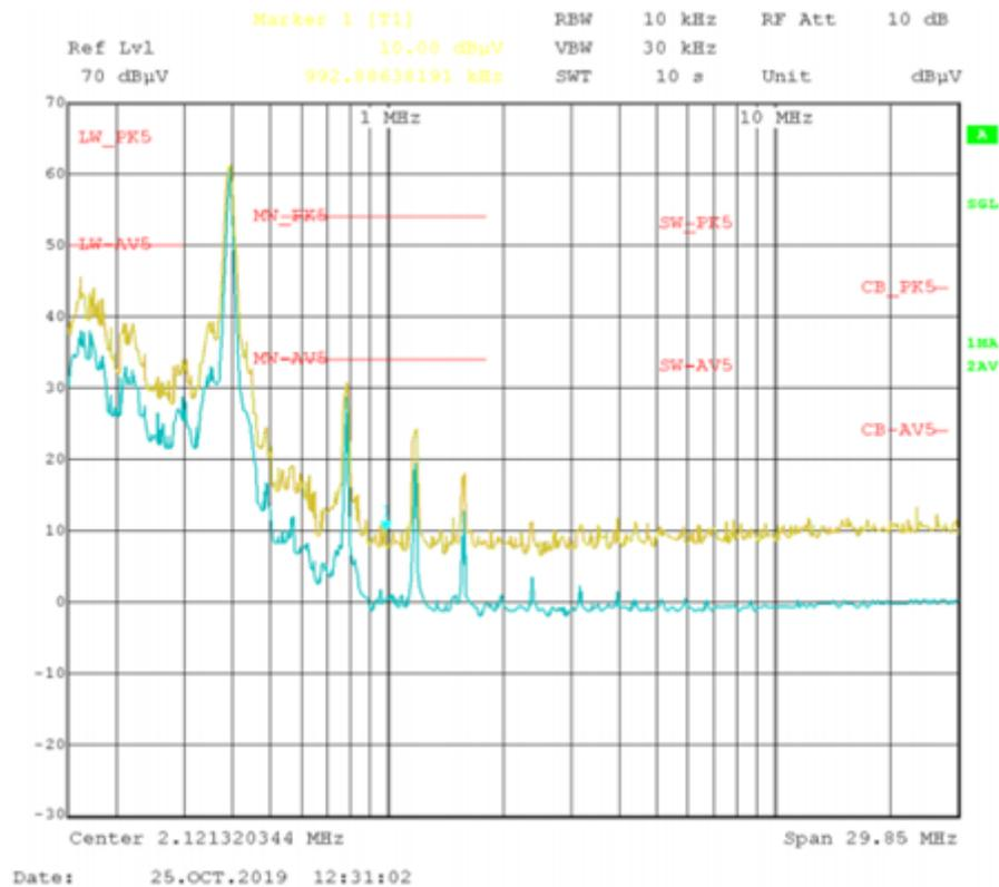
Figure 1. Conducted EMI of the LMQ61460 versus Comité International Spécial des Perturbations Radio 25 (limits: yellow, peak signal; blue: average signal;  $F_{SW} = 400$  kHz;  $V_{OUT} = 5$  V;  $I_{OUT} = 5$  A)
