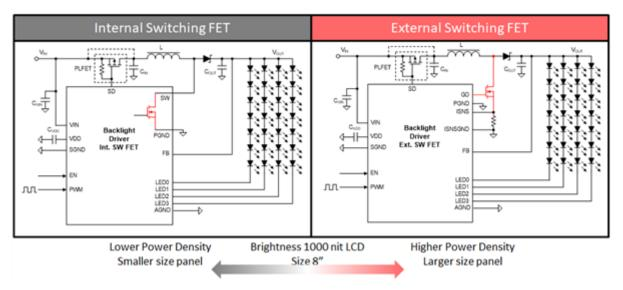
Figure 2. Automotive backlight LED driver topology
