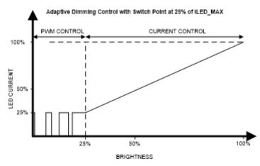
Figure 3. Hybrid dimming mode
