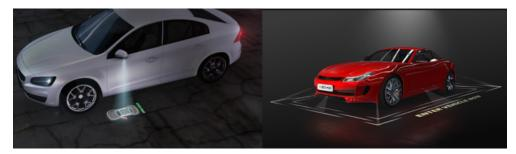
A small lighting module utilizing the automotive grade digital micromirror devices (DMDs), such as the DLP2021-Q1 or DLP3021-Q1, can display an endless number of patterns in any color imaginable. OEMs are not only excited about the styling and customization possibilities features enabled by these products, but also by the possibility of the module to display warnings and alerts to the driver, pedestrians or nearby vehicles.
