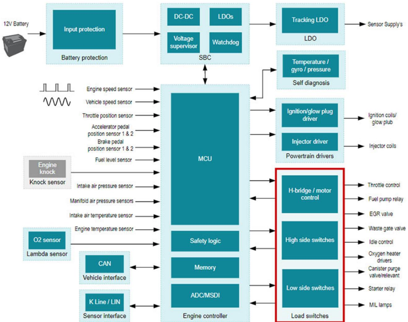
**Figure 2. Block diagram overview of an engine platform design, including input sensors and output load switches (highlighted in red) that interface with the ECU**
