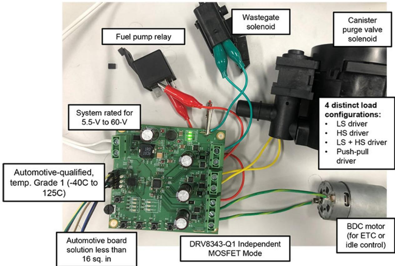
**Figure 5. Engine load interface solution for 12-V and 24-V automotive systems**
