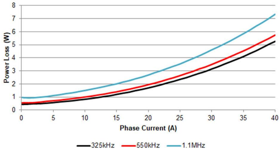
Figure 1. TPS546D24A power loss
