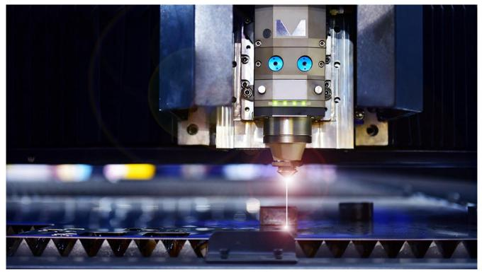
Figure 1. A Laser Cutting Machine
