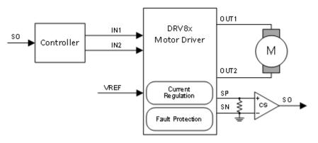
Figure 5. Low-side current sensing approach to stall detection
