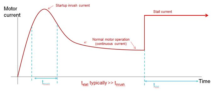
Figure 4. Typical motor current profile during startup (inrush) current, continuous current and stall event current
