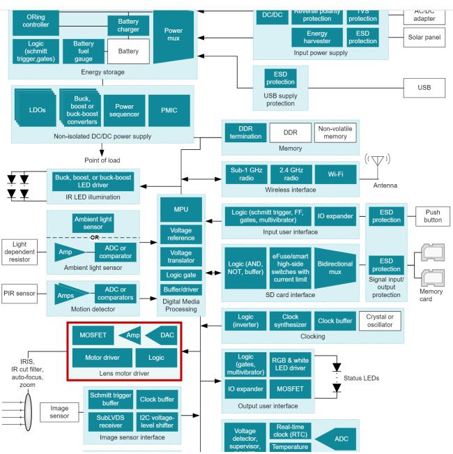
Figure 1. Battery-powered video doorbell system reference design
