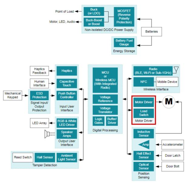
Figure 3. Sections of an electric smart lock
