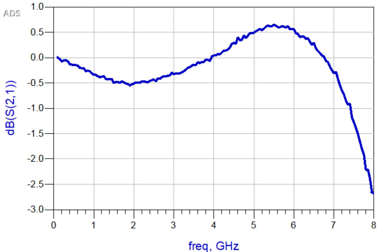
**Figure 2. ADC12DJ3200 Frequency Response Measurement in Dual-channel Mode**
