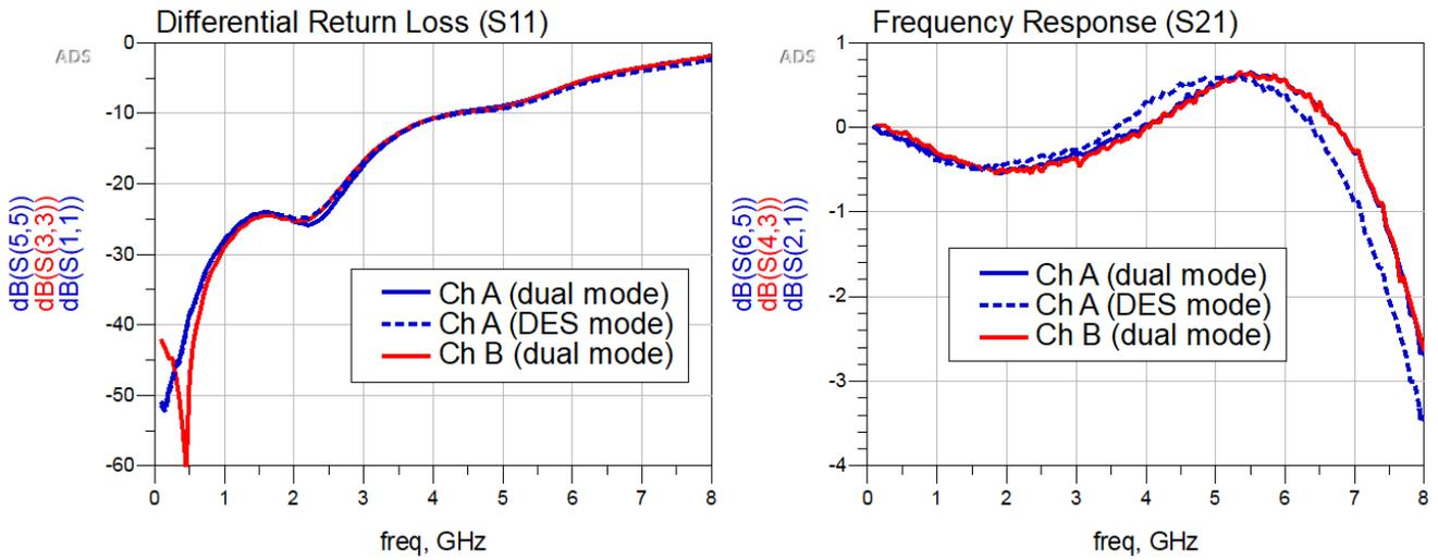
**Figure 5. Final S-parameter Model Simulation Results**
