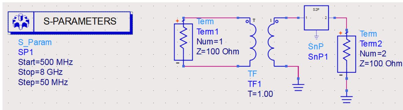
Figure 4. Final S-parameter Model Simulation Setup
