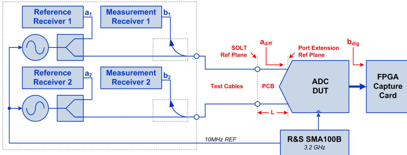
Figure 1. Frequency Response Measurement Setup
