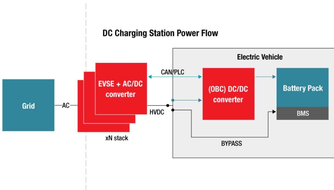
Figure 1. DC Charging Station Architecture
