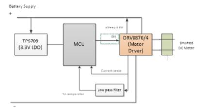
Figure 5. Driving a Unidirectional Motor with the DRV8874 or DRV8876
