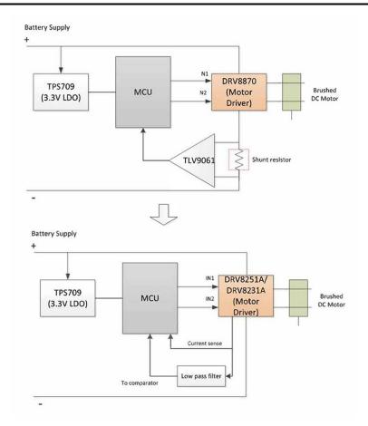
Figure 3. Examples of Driving a Bidirectional Motor, Replacing the DRV8870 with the DRV8251A or DRV8231A
