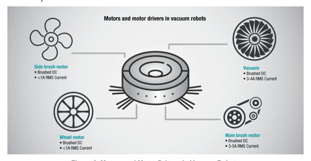
Figure 2. Motors and Motor Drivers in Vacuum Robots
