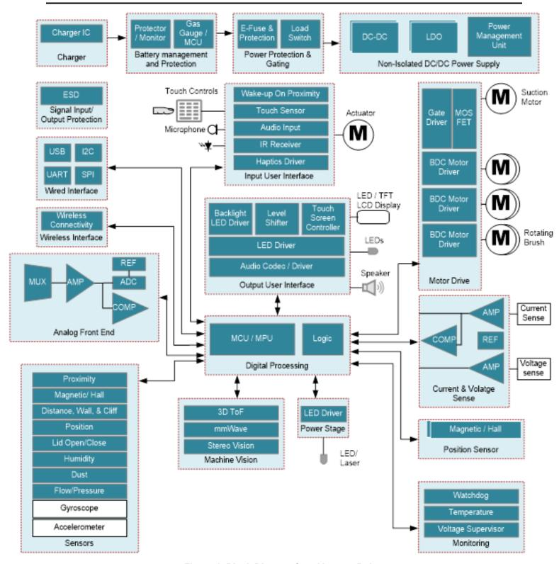
Figure 1. Block Diagram for a Vacuum Robot
