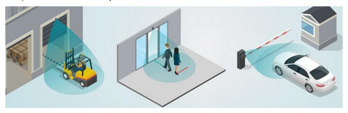
Figure 1. Various automated entrance systems including a) a garage door opening based on vehicle height, b) a sliding door avoiding a false detection and c) an intelligent parking barrier that filters out non-vehicles approaching gate.
