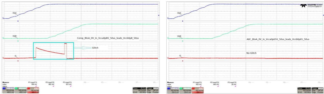
**Figure 3. Glitch Testing Case of a Competing Device (Left) and the SN74AXC1T45 (Right) with a 50-Ms Ramp Rate and 0-v Input**
