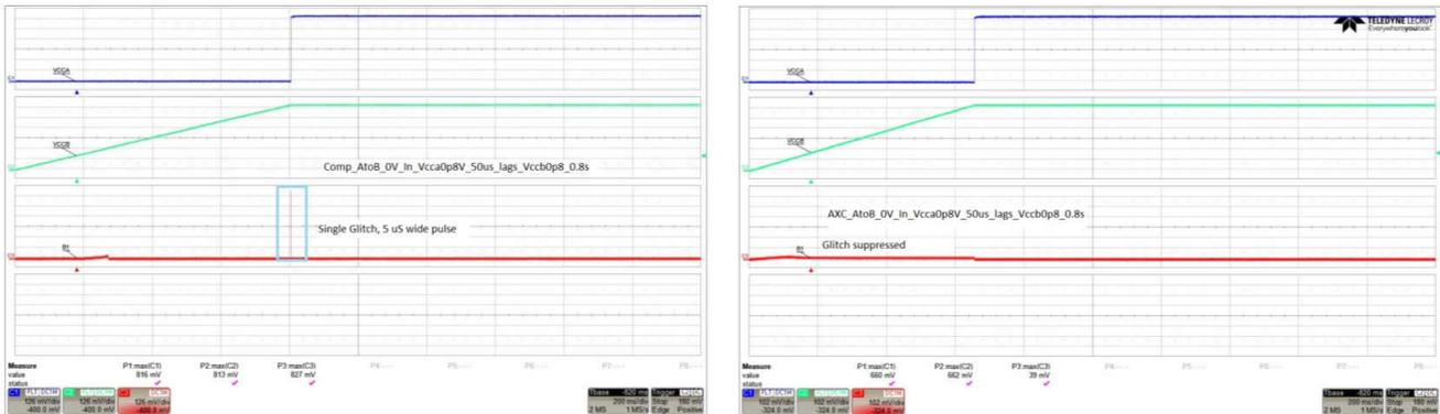
**Figure 4. Glitch Testing Case of a Competing Device (Left) and the SN74AXC1T45 (Right) with 1-s/Vramp Rate and 0-v Input**
