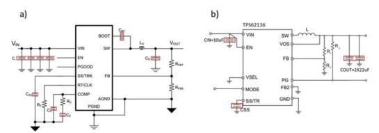
Figure 1. Typical Circuit Schematics for an Externally Compensated Peak-current-mode Control Device (a); and the TPS62136 (b); the Required MLCCs Are Highlighted in Red
