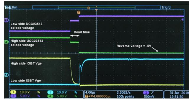
Figure 3. Normal PWM Operation with Interlocking
