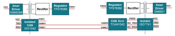
Figure 1. Discrete Implementations of Isolated CAN and Power
