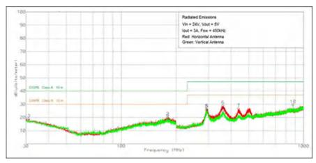
Figure 2. Radiated Emission for the LMZM33603 (5 v Output, 3 a Load)
