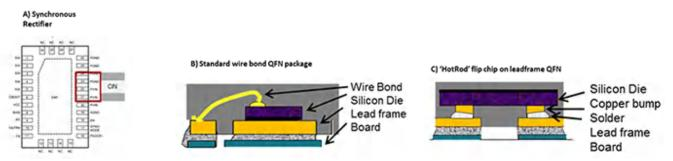
Figure 3. A.QFN Package Capacitor Placement, B.QFN Wire-bond and C. HotRod™ Packaging
