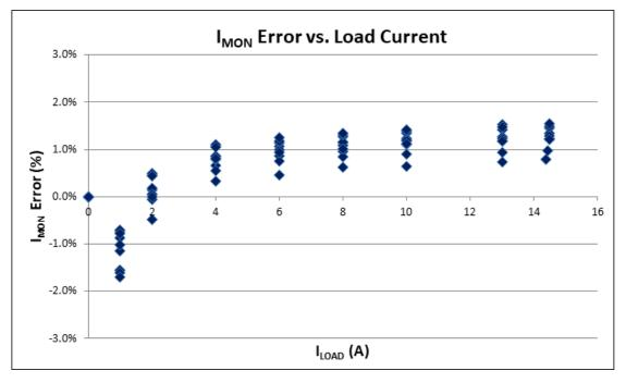
Figure 3. TPS25982 Monitoring Accuracy at Various Currents
