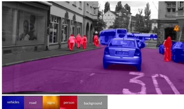
**Figure 1. Classification Example of an Automotive Use Case. Every Object in the Scene Is Determined to Be One of the Five Different Classes.**
