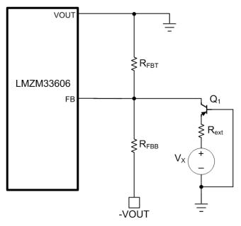
Figure 3. Implementation using a single PNP.
