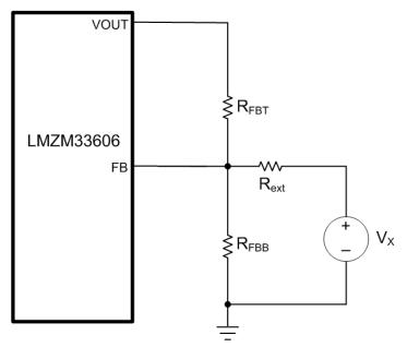
Figure 1. Programmable voltage with a buck topology.
