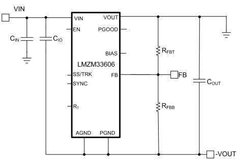
Figure 2. Inverting buck-boost with the LMZM33606.
