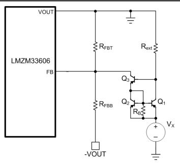
Figure 5. Implementation using a Wilson Current Mirror.
