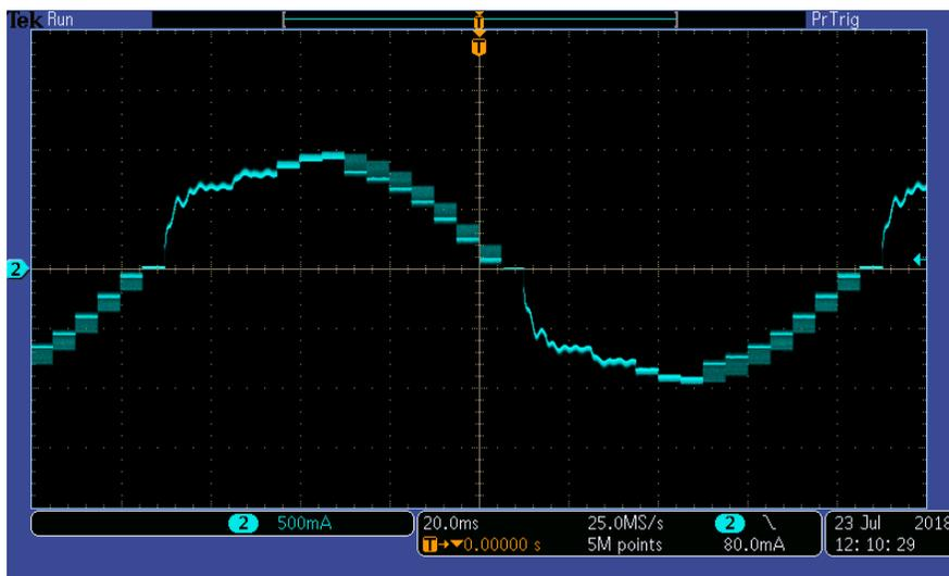
**Figure 4. Stepper Motor Waveform at a Slow Speed (200PPS) with Slow Decay/50% Mixed Decay**
