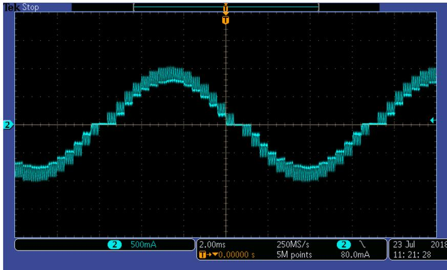
**Figure 2. Stepper Motor Waveform with 60% Fast Decay**
