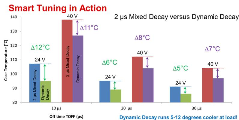
**Figure 7. Dynamic Decay vs. Mixed Decay at Various T<sub>OFF</sub> Times**
