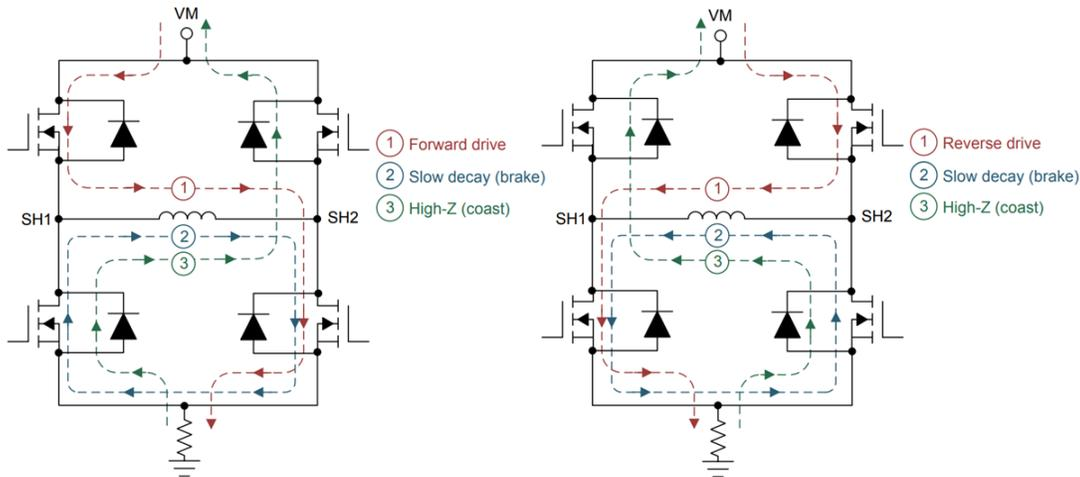
**Figure 5. Current Paths through the H-bridge During Normal Operation (Driving), Dead Time (All FETs Are off), Fast Decay and Slow Decay**
