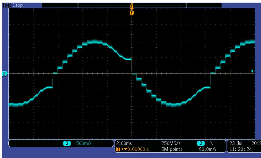
**Figure 3. Stepper Motor Waveform with Slow Decay**
