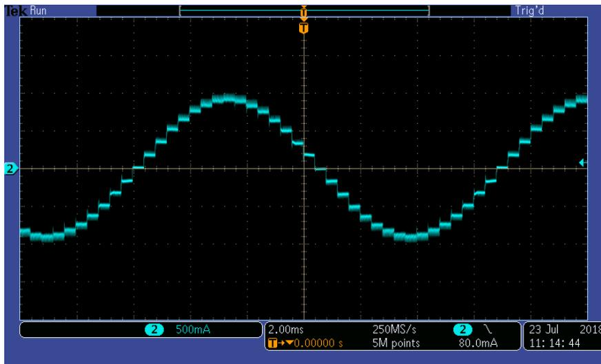
**Figure 1. Stepper Motor Coil Current for a 25V Supply, 2,500 Pulses per Second (PPS) and One-eighth Microstepping Using Ripple Control on the TI DRV8886AT**
