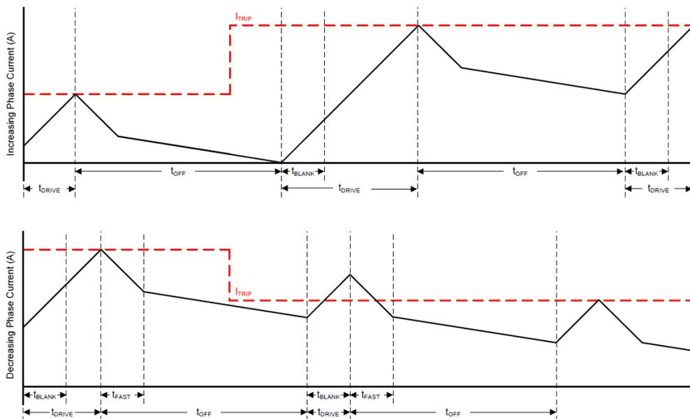
**Figure 6. Using Mixed Decay to Regulate the Current at Each Microstep Level**
