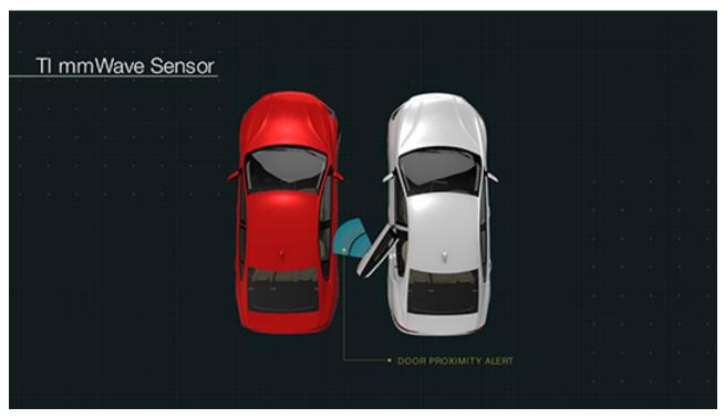
Figure 1. A mmWave Sensor on a Car Door Detects outside Obstacles
