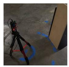
Figure 3. Obstacle Detection Sensor in a Lab Setup, Detecting Wooden Plank
