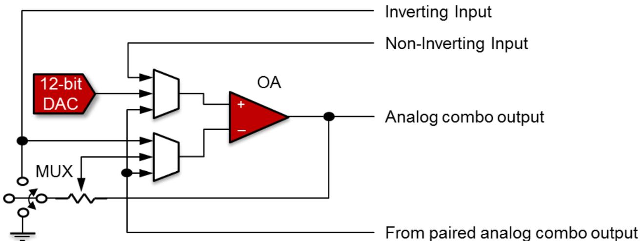
Figure 1. Smart analog combo module diagram
