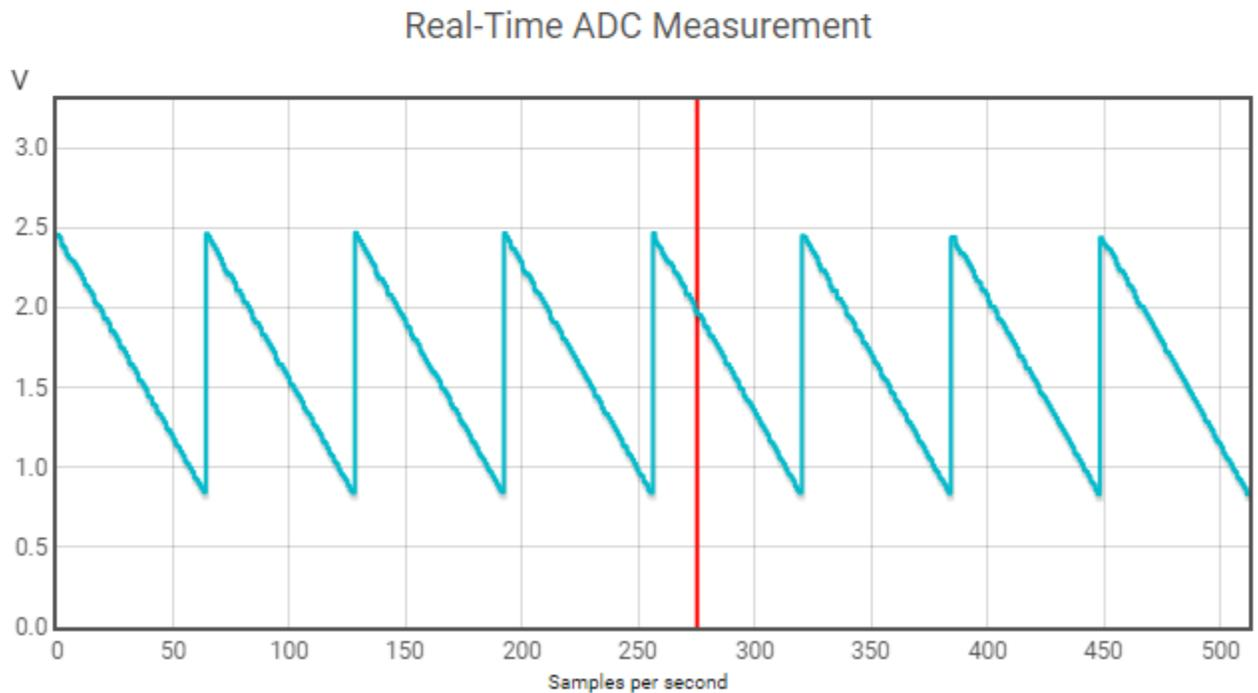
**Figure 7. Sawtooth Inverting Waveform with a Signal Frequency = 8Hz**
