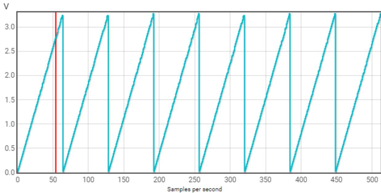
**Figure 8. Sawtooth Noninverting Waveform with Signal Frequency = 8Hz, Op-amp Gain = 2**
