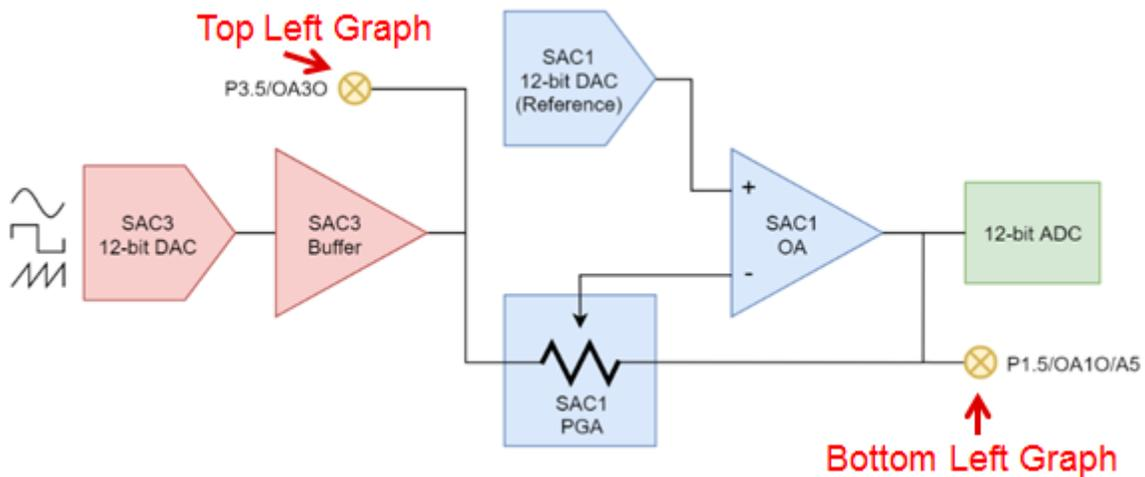
**Figure 6. Smart Analog Combo Modules Block Diagram**
