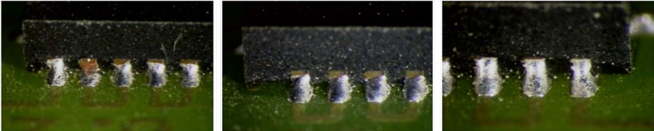
**Figure 2. QFN Package Soldering with Limited Side Wetting and Poor Soldering on One Lead (Left); Limited Side Wetting and Good Soldering (Center); Full Side Wetting and Good Soldering (Right)**
