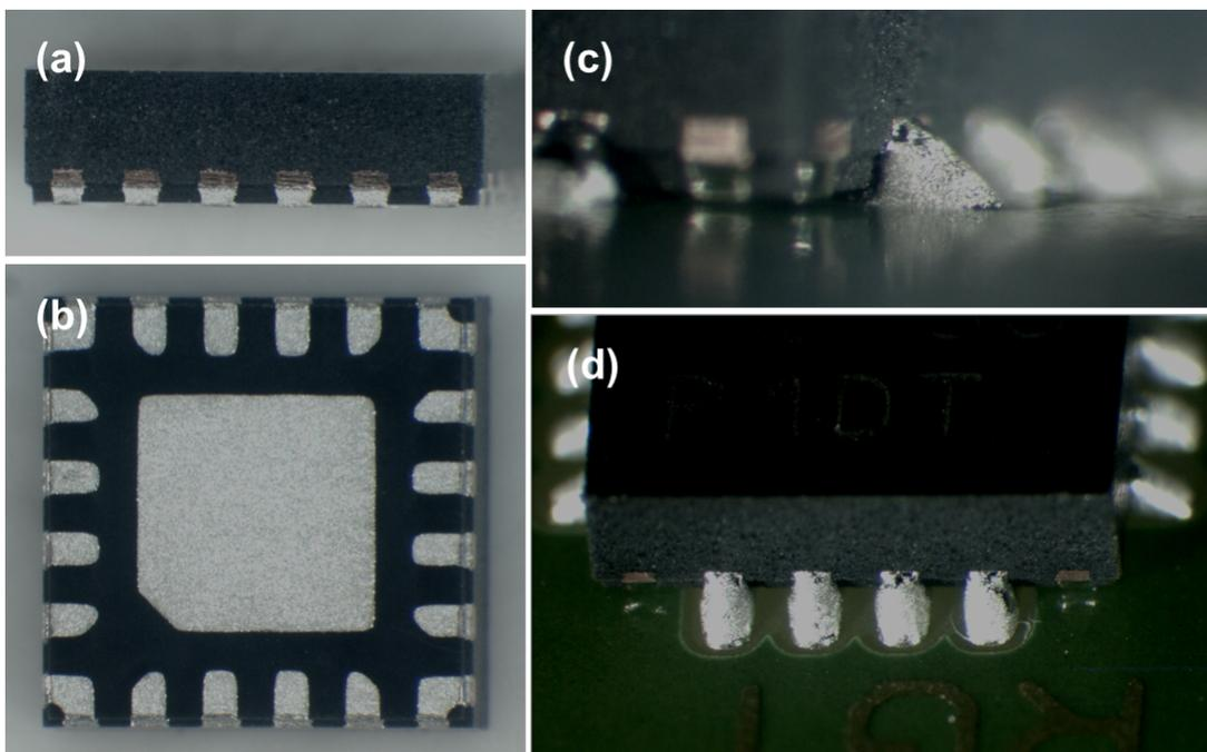
**Figure 3. Side (a) and Bottom (b) View of a QFN Package with Wettable Flanks; Side (c) and Top (d) Views of QFN Package Soldering with Wettable Flanks**
