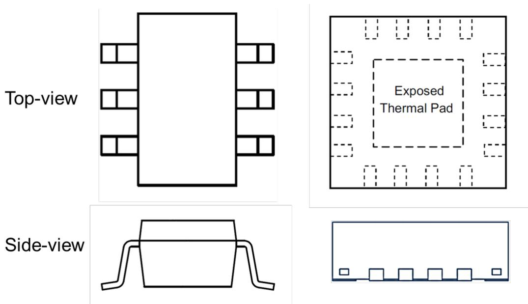
**Figure 1. Package Drawings for SOT (Left) and QFN (Right)**
