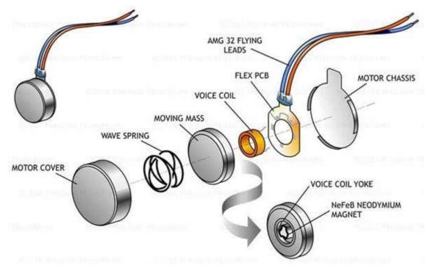
Figure 1. Z-axis LRA (Photo Courtesy Precision Microdrives)
