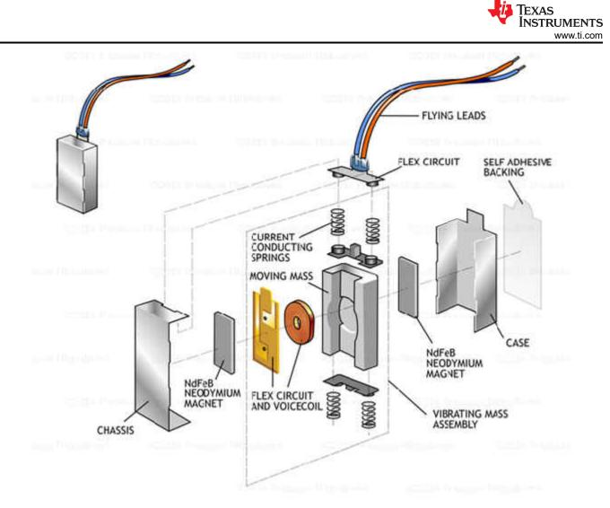
Figure 2. X-axis LRA (Photo Courtesy Precision Microdrives)
