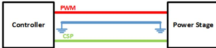
**Figure 5. Optimized Layout Example**
