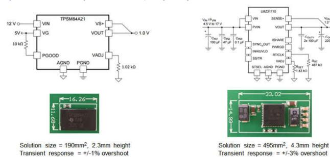
Figure 1. Solution-size Comparison
