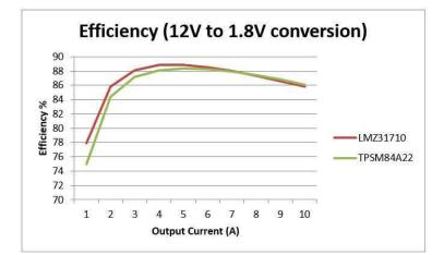
Figure 3. Efficiency Comparison for a 12V-to-1.8V Conversion
