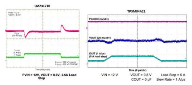
Figure 4. Transient Response Comparison
