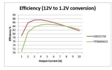
Figure 2. Efficiency Comparison for a 12V-to-1.2V Conversion
