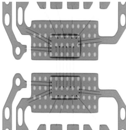
**Figure 1. High Voltage Isolation Multi-chip Module**
