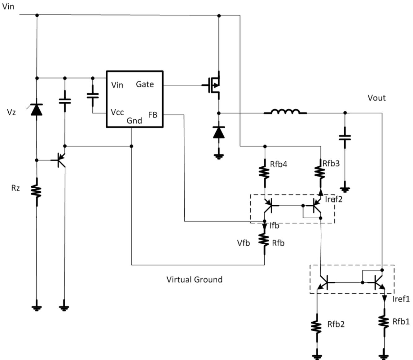
**Figure 5. High-level Schematic of a Nonsynchronous Controller and Feedback Implementation Using Matched-pair Transistors**
