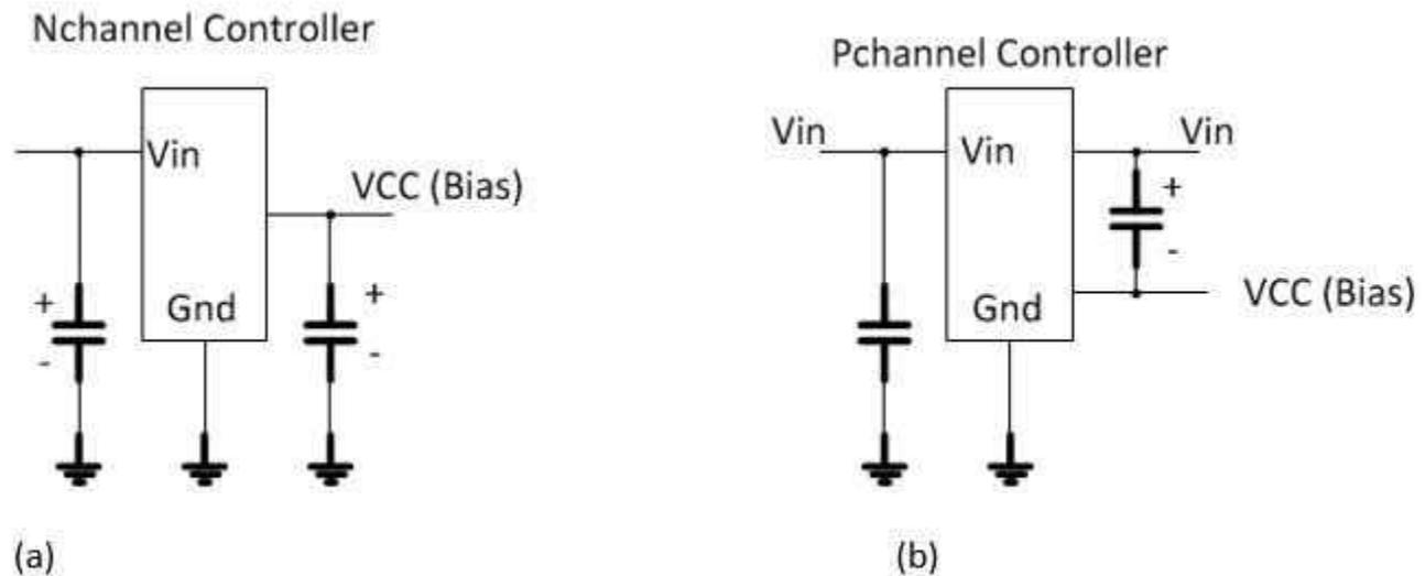
Figure 1. VCC Bias Generation for N-channel (a); and P-channel Controllers (b)
