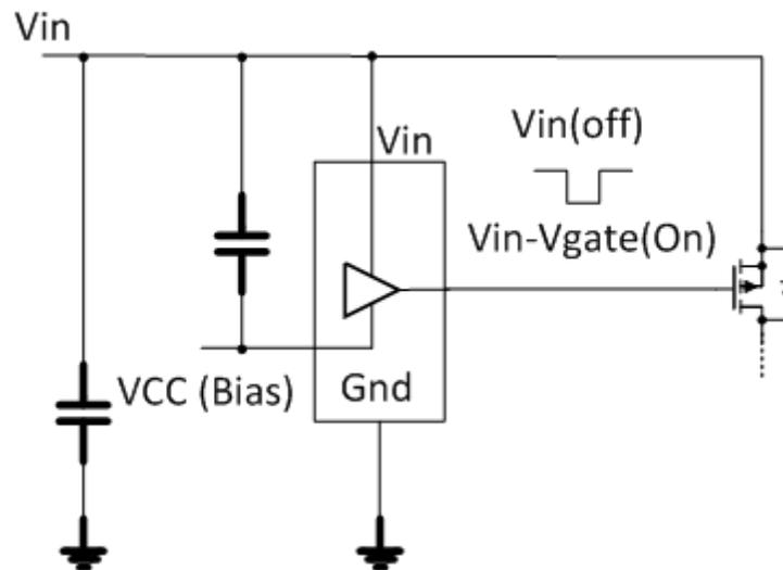
**Figure 2. Gate Drive for a P-Channel Controller**
