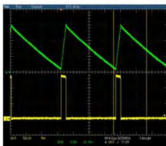
Figure 8. Channel 1 Switch-node Voltage, Channel 4 Inductor Ripple Current
