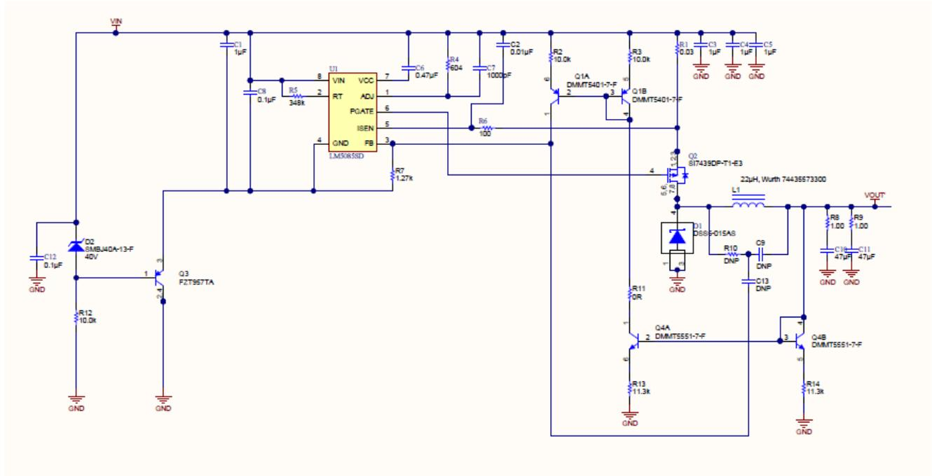
Figure 6. A 24V to 150V<sub>IN</sub> (Max)/12V<sub>OUT</sub> At 3A Design Using the LM5085
