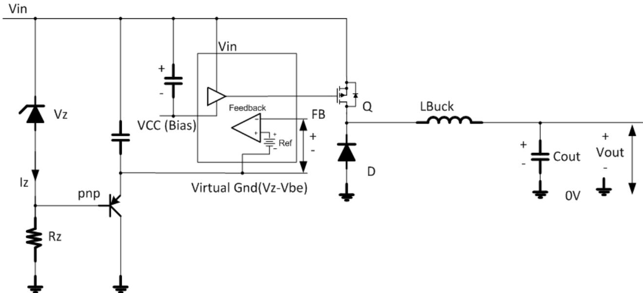
Figure 4. Schematic Showing the Difference in Voltage Potential between  $v_{OUT}$  (Referenced to 0V Ground) and the Feedback Voltage of a Controller (Referenced to Virtual Ground)
