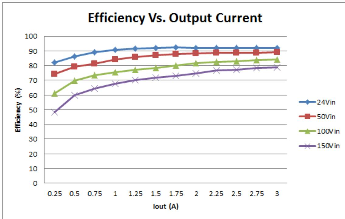
Figure 7. Efficiency (%) vs. Load Current (a) at Various Input Voltages
