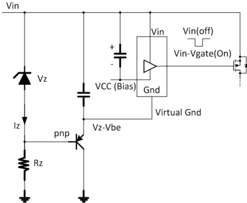
Figure 3. Creating a Virtual Ground Using a Simple Emitter Follower Scheme
