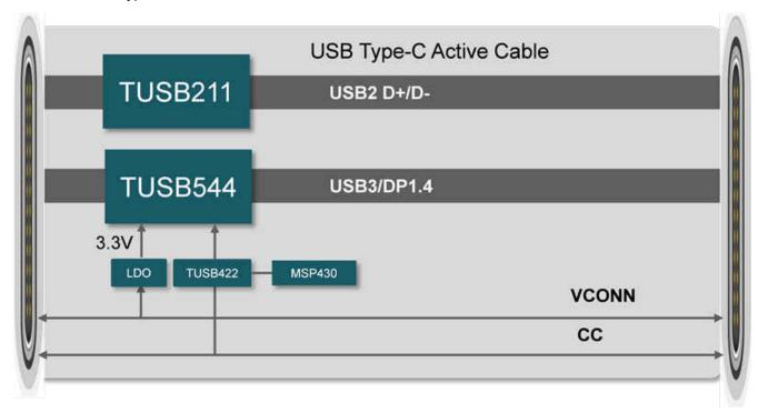
Figure 3. USB Type-C Active Cable Solution with the TUSB544 And TUSB211
