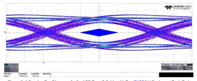
Figure 5. A Passing Eye Diagram of a 5m USB Type-C Cable with Two TUSB544 Devices at Each End
