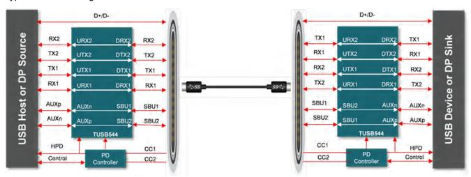
Figure 1. Enabling Better Signal Quality with the TUSB544 as an End-to-end Solution
