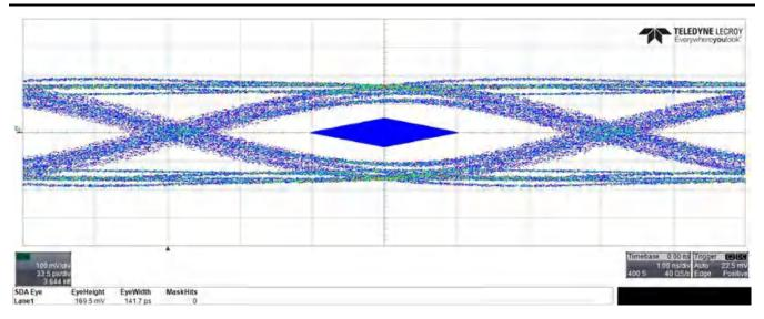
Figure 4. A Passing Eye Diagram with the TUSB544 Inside a 3m USB Type-C Cable
