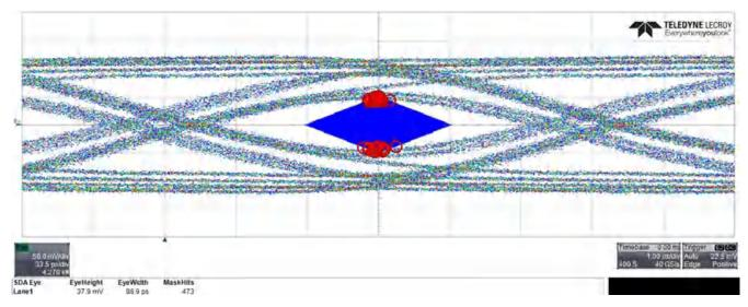
Figure 2. A 3m USB Type-C Cable Failing the Eye Diagram
