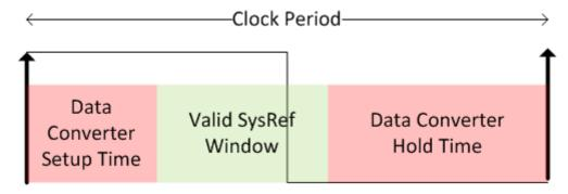
Figure 1. SysRef Pulse Edge Placement
