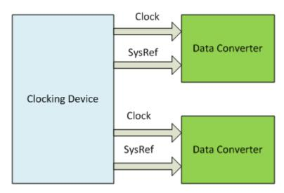
Figure 2. Single Clocking Device Approach
