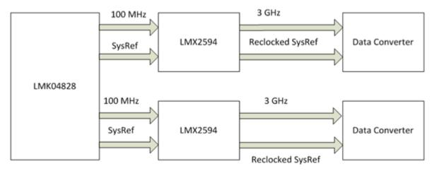
Figure 4. High-speed Clocking Example
